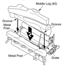
Figure 22 - Installing Middle Log (#2) [18" Variable Manually-Controlled Set Shown]
